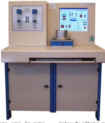
The spark test apparatus serves for testing intrinsically safe circuits. The test is based on whether the tested equipment is capable of producing sparks, arcs in normal operation, capable of igniting the gas mixture specified by the standard, in the given chamber, under given conditions.
